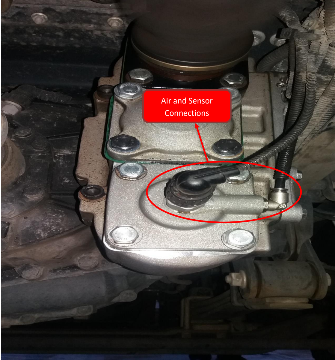
Figure 5 – Picture of Air and Sensor Wire Connections
