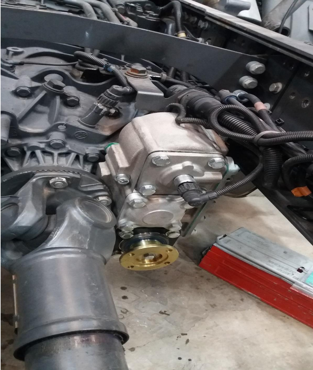
Figure 4 – Assembled sample ZF.11 PTO
